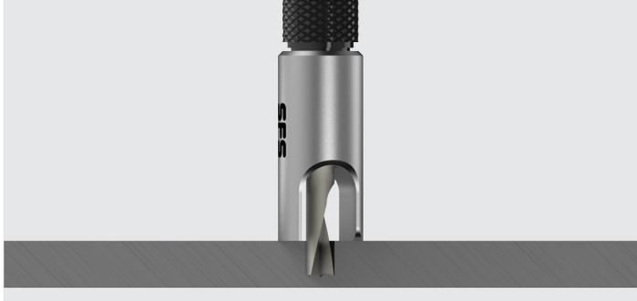
The geometry of the drill hole shall be checked minimum on 1% of all drillings. **Nominal measure: Ø 5,9 – 6,0 mm**
