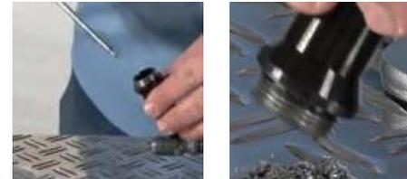
4. Open the jaw mechanism with two wrenches: PowerBird® Pro & AccuBird® Pro – use 2 x 17mm wrenches; PowerBird® & Accubird® – use a 14mm and 17mm wrench.
