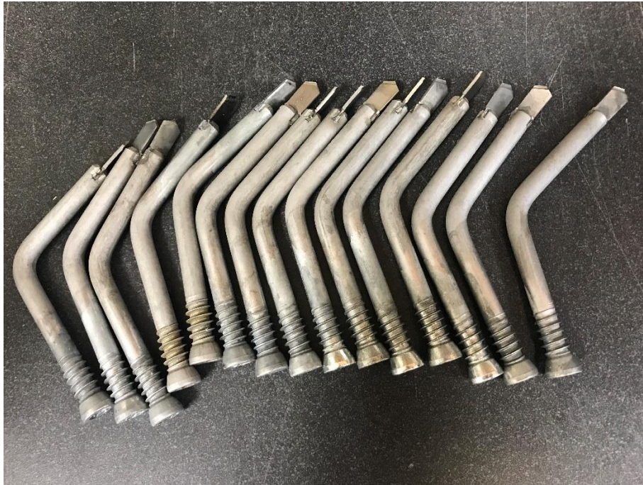
Photo No. 4 Coating Stripped for Base Metal Root Diameter Measurement
